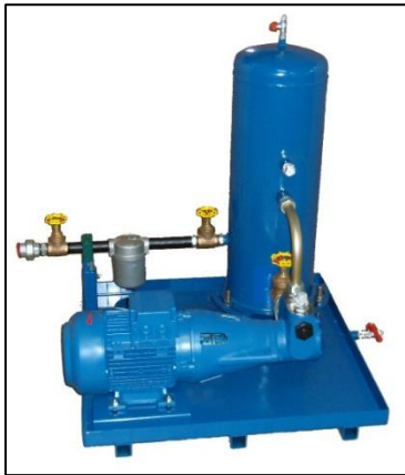
Figure 16 The oil buffer tank
