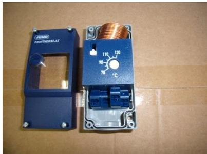
Figure 26 – Thermostat maximal
