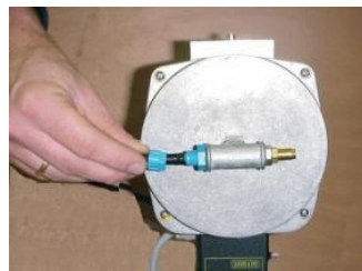
Figure 11 Connecting the air pressure sensor
