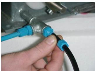
Figure 11 Connecting the air pressure sensor
