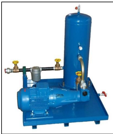
Figure 16 The oil buffer tank
