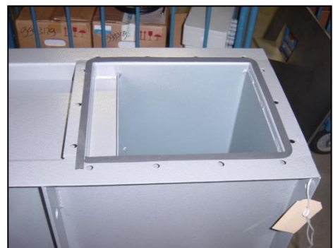
Figure 7 sealing tape application
